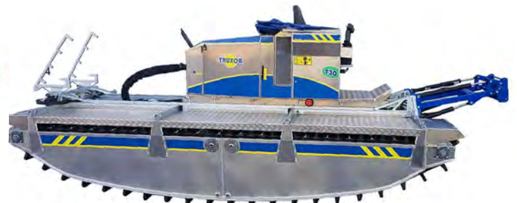
The movable driver's cab is hydraulically adjusted and works as counterweight during heavy lifts in water.
