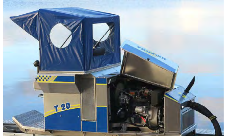
Easily accessible engine compartment facilitates service.
